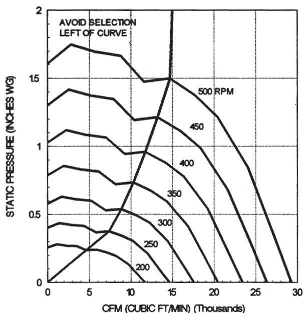
Performance certified is for installation type A - free inlet, free outlet.
