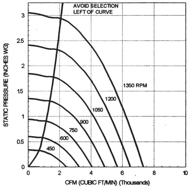
Performance certified is for installation type A - free inlet, free outlet.
