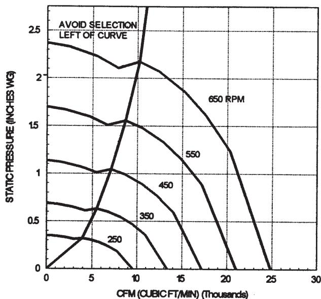
Performance certified is for installation type A - free inlet, free outlet.
