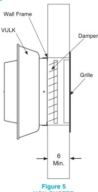
Figure 5 NON-DUCTED Sidewall Installation
