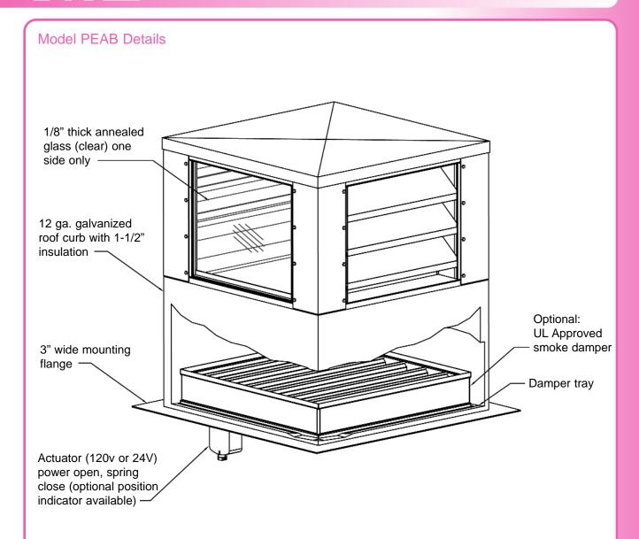
The Carnes Company is pleased to announce our newest product addition - the PEAB louvered penthouse elevator vent assembly. Designed with three louvered sides and one side of 1/8" annealed glass, the PEAB assembly is built specifically for ventilation and emergency smoke evacuation of elevator shafts.
