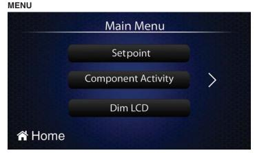
The "Menu" page displays four features: Setpoint, Component Activity, Dim LCD and Help. Tapping any of
