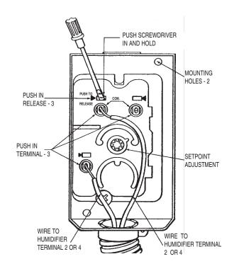
The control should be located in the duct where it will be affected by normal air flow. The control can be mounted in any position, but where possible locate it on the side of the duct to make the setpoint adjustment easily accessible.
