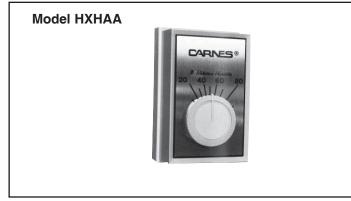
Mount this humidistat four or five feet above the floor in freely circulating air of the temperature and humidity about average for the entire space to be controlled. Avoid locations near hot or cold air ducts and discharge air from the humidifier. Scale range is from 10-90% RH. Differential is 5% non-adjustable.
