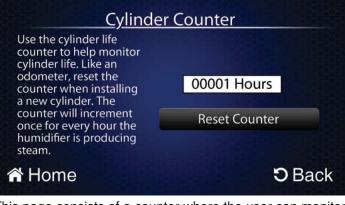
This page consists of a counter where the user can monitor the life, in hours, of the cylinder. When changing a cylinder, press the 'Reset' button on this page to reset the timer. The Cylinder Life Counter only counts the amount of actual runtime of the cylinder (the time when the contactor is pulled in). The counter value is saved even when the humidifier is powered down. The national average cylinder life is about 1150 hours, but this can vary greatly depending on individual water conditions.
