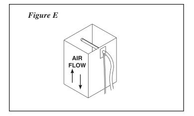
The distributor pipe should be located to insure best distribution of steam into the airstream. A minimum clearance of 4" must be maintained between the top of the duct and the distributor pipe.
