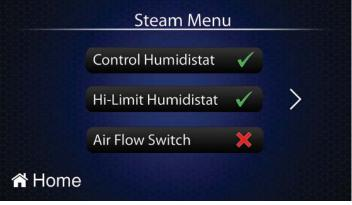
The "Steam" menu page will display the status of the four basic controls (Control Humidistat, Hi-Limit Humidistat, Air Flow Switch and Door Interlock). The humidifier will only produce steam when the unit is switched into the "ON" position, and if all four controls are satisfied.
