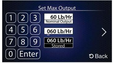
The maximum steam output of the unit can be set on this page. The maximum output value cannot exceed the nominal output value of the unit, and it cannot be set below 20% of the nominal output. The nominal output of the unit is listed on the nameplate and the previous screen.
