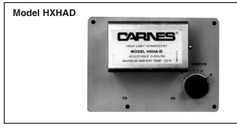
The Model HXHAD is available to reduce the potential of condensation occurring in the supply duct. The control must be mounted a minimum of 10 feet downsteam of the steam distributor pipe. Setpoint range is 15-95% RH. Differential is 5% non-adjustable.
