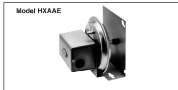
Air flow in the duct may be sensed by using this differential pressure switch. The differential in pressure between the interior of the duct closes a switch when air is moving. Air pressure differential as low as .07 w.g. may be sensed with this switch. **Environment:**
