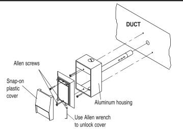
Remove any excess insulation from the duct that would prevent the probe from extending a minimum of 4" (106mm) into the air stream.
