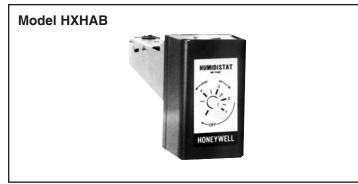
This duct mounted humidistat is installed in the return air duct to sense the humidity level in the area being served. Scale range is 15-50% RH. Differential is 4-6% non-adjustable.
