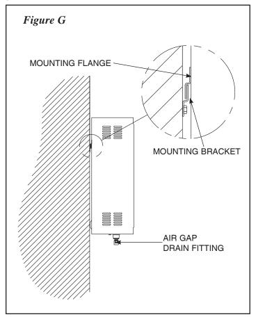
Place the mounting flange on the humidifier cabinet over the mounting bracket. A sheet metal screw should be installed through the back of the humidifier cabinet to secure the humidifier to the mounting bracket.
