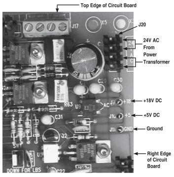
5. If 24V AC is not present reset the overload located on the transformer and recheck. If the transformer in your humidifier does not have a integral overload breaker as shown below, check the inline fuse in the adaptor harness. If necessary replace with type 2AG - 3 amp (slow blow).
