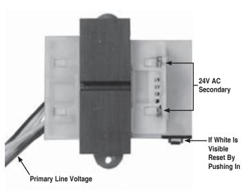
6. If 24V AC is present the electronic control board may be defective.
