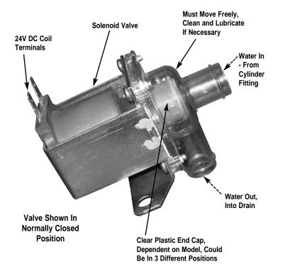
The "Drain Solenoid" LED indicates if the electronic circuit board is sending 24V DC to the valve. If the LED is off but 24V DC is present at the drain solenoid coil the circuit board may be defective.
