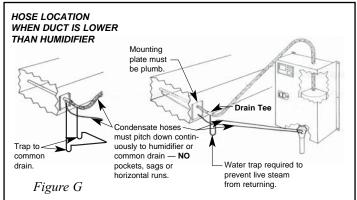
It is very important that both the steam hose and condensate return line, whether flexible or hard tubing, be installed so there are no sags, low points, dips or horizontal runs. The steam is at a very low pressure and it cannot overcome any resistance caused by accumulating water standing in the steam hose. Accumulation in the condensate return hose will hamper the flow and may cause water to enter the duct work by way of back up in distributor pipe.
