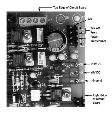
5. If 24V AC is not present reset the overload located on the transformer and recheck.
