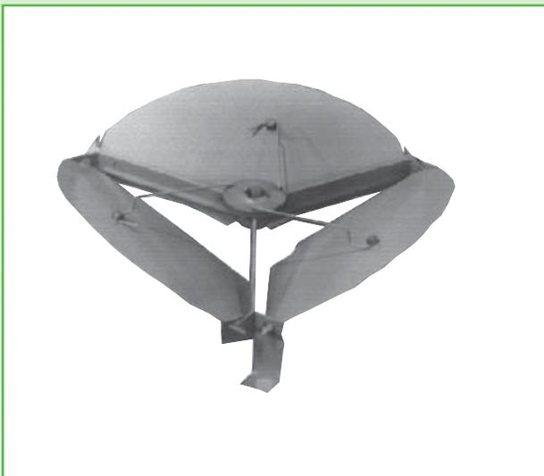
The model KXMB volume control dampers are opposed blade, gang operated, fully adjustable units. The opposed blade action distributes air evenly over the diffuser. Model KXMB dampers are installed in the neck of the diffuser.
