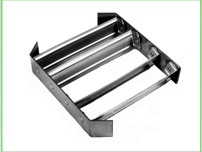
The model KXYA equalizing deflector is a grid to equalize the air flow through a stub duct to the diffuser. Recommended installation is flush with the duct take-off collar. Each blade is individually adjusted to any position desired. The end tabs hold the grid in place by friction.
