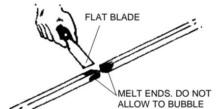
5. Remove the tool and immediately push the belt ends together. The softened material should flow slightly out of the joint, but do not squeeze all of the melted material out. Hold together for 2 minutes. If material bubbles, it is too hot and will not maintain the bond. Retrim and re-weld at a lower temperature.
