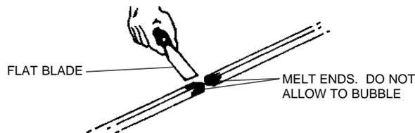
2. Remove the tool and immediately push the belt ends together. The softened material should flow slightly out of the joint, but do not squeeze all of the melted material out. Hold together for 3 minutes. If the material bubbles, it is too hot and will not maintain the bond. Re-trim and re-weld at a lower temperature.
