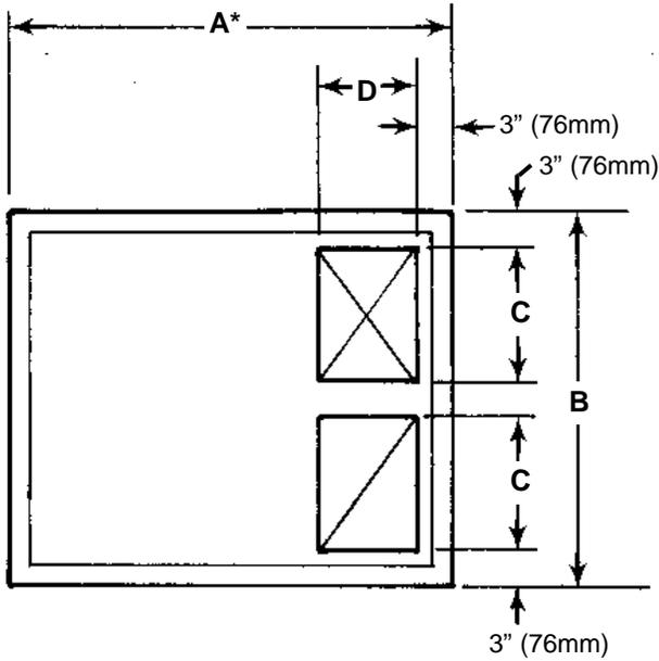
**NOTE:** Allow at least 24" (610mm) clearance on all sides of the unit, except for the control panel side for servicing. You must allow enough room around the control panel to meet local codes concerning serviceability.
