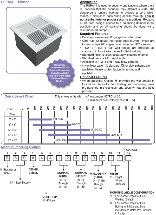
DIMENSIONAL DATA | Sleeved Security Ceiling Diffuser, Suicide Deterrent Core
