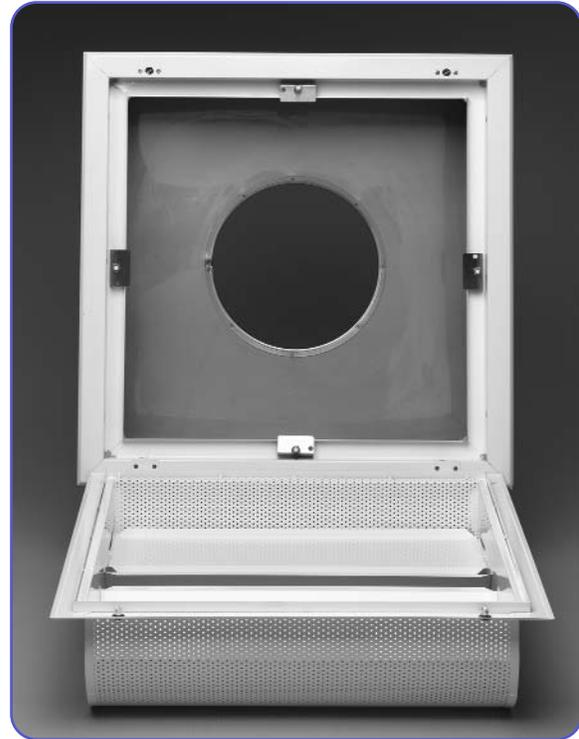
The Carnes DD Series Radial Flow Diffuser has been designed to provide low aspiration and high ventilation rates especially for clean room applications such as research laboratories, animal labs, food processing, hospital rooms and computer rooms. The unique design of solid baffles in an intrusive perforated face can handle large volumes of air with low initial face velocities.
