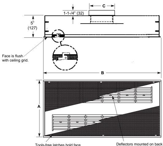
Tools-free latches hold face assembly to ceiling plate assembly.
