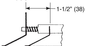
Two spring-loaded pins, four-pin suspension to ceiling plate.
